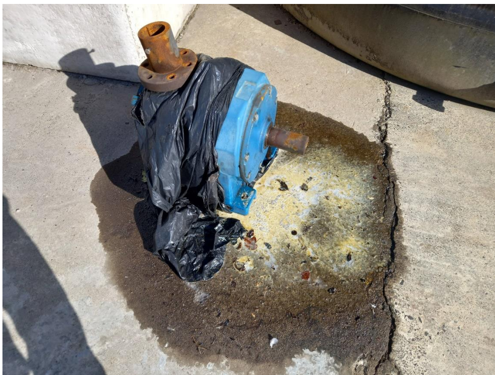
Photograph 19: Oil-leaking machine part
